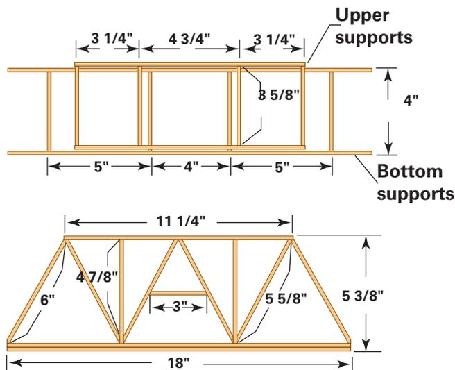
4. Your design must be able to fit the piece of hardwood used to test the bridge. Leave an opening that measures at least  $1\frac{1}{2} \times \frac{1}{2}$  inches across the middle of your bridge. This is where the hardwood and bucket will fit.
